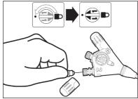
Unscrew cap #3 and pull release wire 3-4 cm or until tension is felt.
